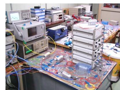
Commercial optical MUX's, optical amps,
