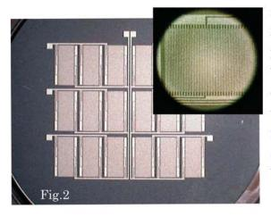
inducing coherently-additive emission from more than 2000 photoconductive emitters using an ultra-short pulse Kr\*F laser (Fig.2).
