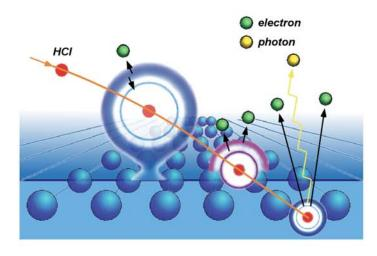
Left: Interaction of an HCI with a solid surface. The huge potential energy of a HCI induces nano-scale modification on a surface.
