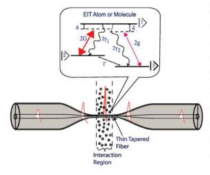
prepare a very thin part with a subwavelength diameter along the fiber. Left figure illustrates a schematic diagram. The very thin part is embedded in an optical medium. Light propagating in the fiber interacts with the medium through evanescent field in the very thin region. We can manipulate quantum coherence of the medium through the evanescent field and can control the quantum optical behaviors of the propagating light.
