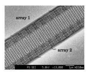
Fig. 1 Capacitively coupled arrays of small Josephson junctions. Each array is composed of serially connected parallel two-junctions pairs.
