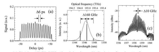
(a), (b): 1.5-ps, 168-GHz DISC-gating window shape and its Fourier-transformed spectrum\*)
