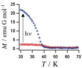
Figure 1. Photo-induced magnetization of a [Fe(N<sub>3</sub>)<sub>2</sub>(pyrimidine)]-based antiferromagnet with  $T_N = 39$  K.
