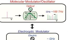
We have realized that by driving Raman processes adiabatically a high density molecular ensemble ( $\sim 10^{20}$  cm<sup>-3</sup>) can be made to coherently vibrate and/or rotate. Such a molecular ensemble can be applied to a light modulator at ultra-high frequencies of  $\sim$  GHz  $\sim$  100 THz.
