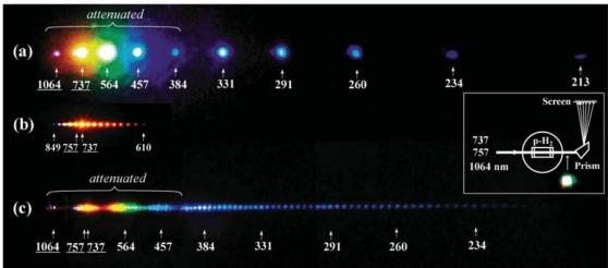
All of the sideband radiations are of a high quality as an actual coherent light source over infrared to near vacuum-ultraviolet wavelengths. We believe this process to be applied as a novel ultra-short pulse laser using these light sources, in which center frequencies and repetition rates are widely tunable.
