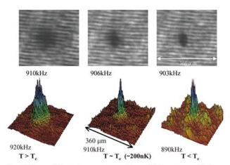
Fig.1 Bose-Einstein condensation of Rb atoms. Below a critical temperature  $(T_c)$ , a narrow peak appears in the velocity distribution of atoms.
