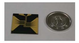
Fig.2 Atom chip (micro integrated atom circuit). Gold wires are fabricated on a Si substrate. Magnetic waveguide potentials for cold atoms can be generated by flowing current through wires.
