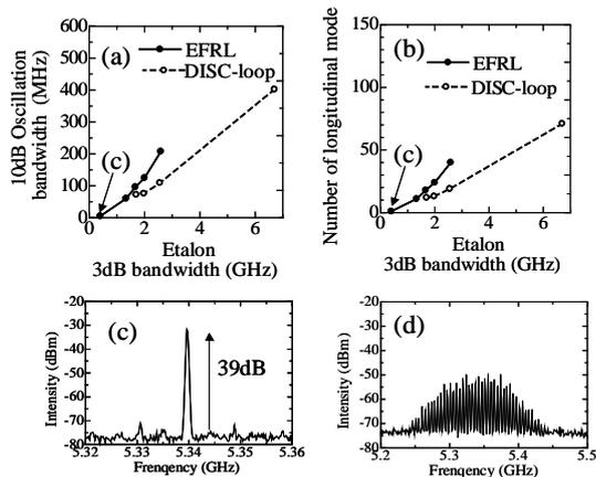
Fig. 5. (a):Comparison EFRL oscillation bandwidth and DISC-loop one. (b):Comparison EFRL number of longitudinal mode and DISC-loop one. (c):RF spectrum using etalon-#a (3dB bandwidth =430MHz) (d):RF spectrum using etalon-#b (3dB bandwidth = 2.0GHz)
