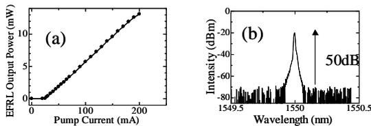
Fig. 4 : (a) EFRL output characteristic using etalon-#a, threshold pump current = 28mA (threshold pump power = 10mW) (b): EFRL output spectrum, pump current = 60mA (pump power = 31mW, Total gain = threshold + 15dB)
