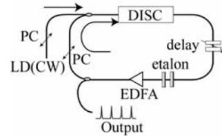
Fig. 2: DISC-loop type pulse generator
