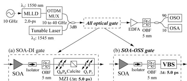
Fig. 3. Experimental setups of the two alternative all-optical gate schemes.
