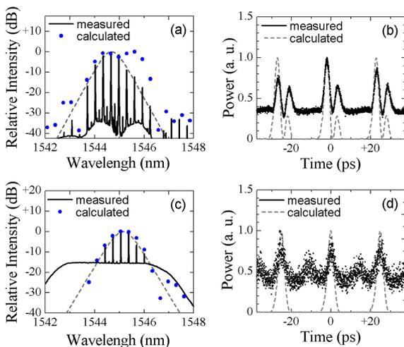
Fig. 4. Measured (solid) and calculated (dotted, dashed) optical spectra and waveforms at the output of all-optical gates with 2.0-ps, 40-GHz, 41-fJ clock input pulses.
