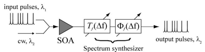
Fig. 2. The new scheme of our all-optical gate which contains an optical spectrum's phase-and-amplitude synthesizer<sup>8</sup>.
