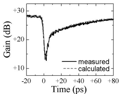
Fig. 1. Measured (solid) and calculated (dashed) SOA gain recoveries of a standard SOA (which differs from the SOA in Sections 2 and 3), after it amplified a 1.25-GHz, 2.1-ps, 8-fJ input pulse. The first- and second-slowest recovery time constants were 54 ps and 6.5 ps, respectively.
