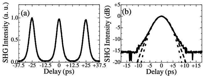
Fig.2. Autocorrelation trace of 40-GHz, 4.5-ps pulse train.
