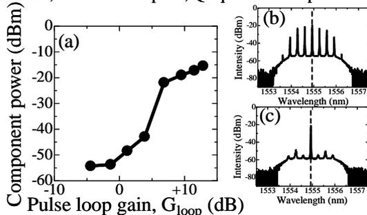
Fig.3. Threshold condition for pulse generation.
