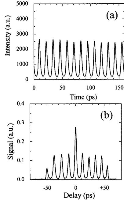
Fig. 4. 84-Gb/s data pulses at the input: (a) averaged image with a streak camera and (b) autocorrelation trace.
