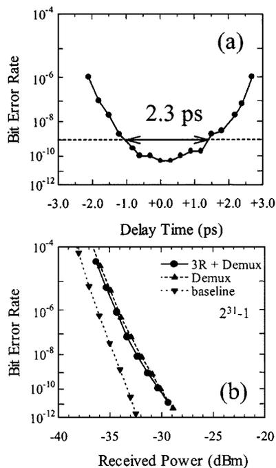
Fig. 6. Error rates of the regenerated pulses.
