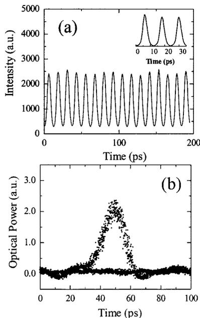
Fig. 5. Regenerated data pulses: (a) streak camera images of the regenerated 84-Gb/s pulses and (b) eye diagram of the regenerated-and-demultiplexed 10.5-Gb/s pulses.
