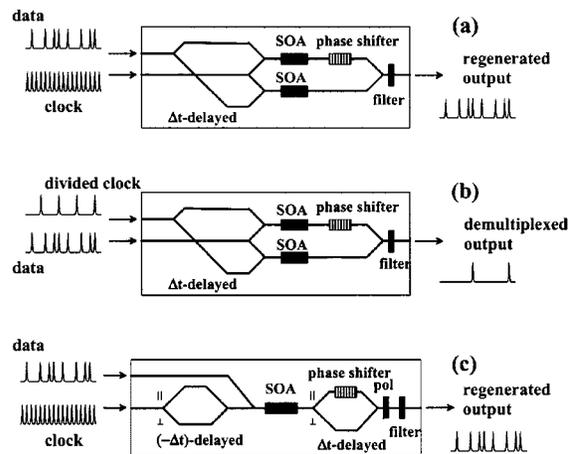
Fig. 1. SMZ-type all-optical device structures: (a) 3R regenerator scheme with SMZ structure, (b) demultiplexer scheme with SMZ structure, and (c) 3R regenerator scheme with PD-SMZ structure.
