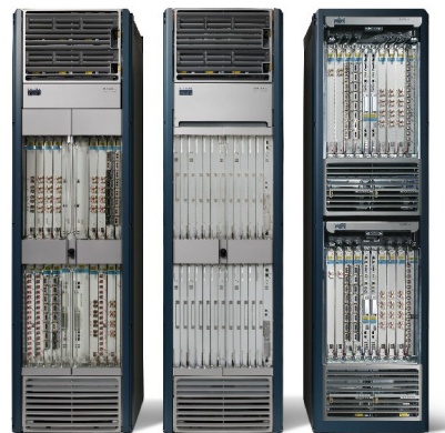
Fig. 2: A part of the Cisco's 92-Tb/s high-end router, CRS-1 (Ref. 4).
