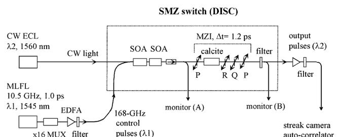
Fig. 1. Experimental Setup: 168 GHz 1.0 ps 1545 nm control pulses modulate 1560 nm CW light through all-optical SMZ switch (DISC configuration). SOA (nonlinear element) consists of two cascaded SOA modules.
