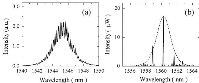
Fig. 4. Comparison of optical spectrum qualities of 168 GHz pulses (a) 1545 nm control pulses, and (b) 1560 nm output pulses (dashed curve shows calculated spectrum of transform-limited 1.2 ps pulses).
