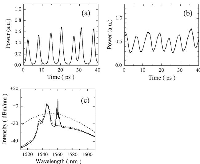
Fig. 2. Optical components before and after cascaded SOAs (a) 168 GHz 1545 nm control pulses, (b) 1560 nm component at SOA output, (c) optical spectra at SOA output.
