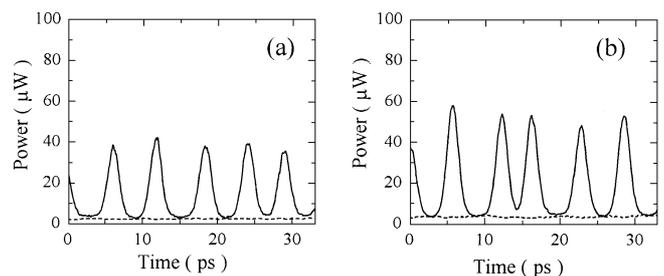
Fig. 3. All-optically switched 1560 nm component at switch output 168 GHz control pulse energies were (a) 10 fJ (average power = 1.7 mW) and (b) 1 fJ (170  $\mu$ W).
