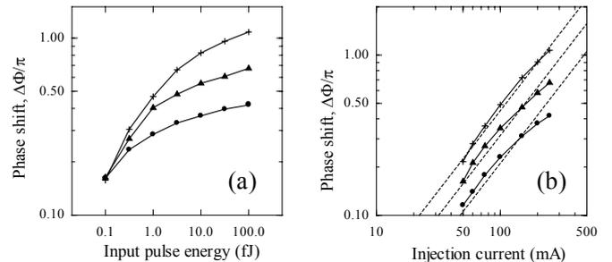
Fig. 5 Measured nonlinear phase shifts as functions of the input pulse energy and the injection current to the SOA. The input pulse frequencies were 168 GHz (circles), 84 GHz (triangles), and 42 GHz (crosses).
