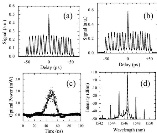
Fig. 4 Wavelength conversion at 168 Gb/s. Autocorrelation trace for the input random pulses (a), that of the output random pulses
