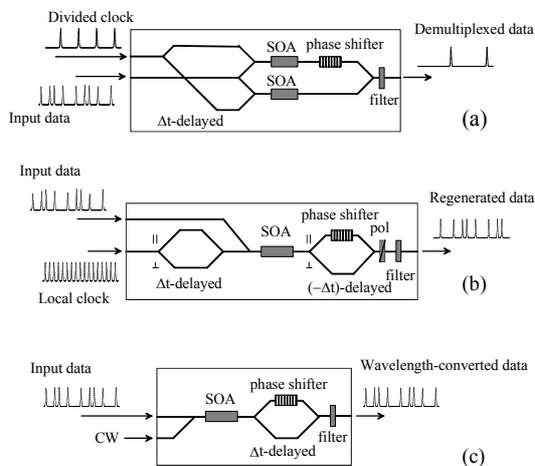
Fig. 1 Three configurations of SMZ-type all-optical switches. (a) original SMZ switch [1] for demultiplexing, (b) PD-SMZ switch [2] for regeneration, and (c) SMZ-DISC [3] for wavelength conversion.
