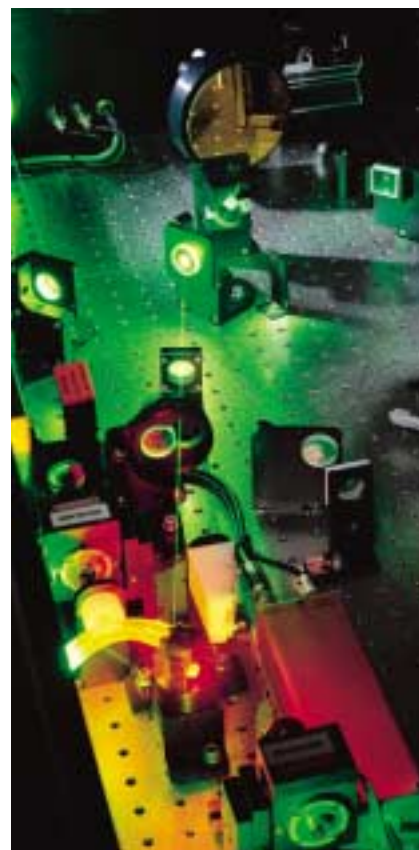
Regenerative amplifiers such as the Spitfire deliver higher pulse energies at lower repetition rates.
